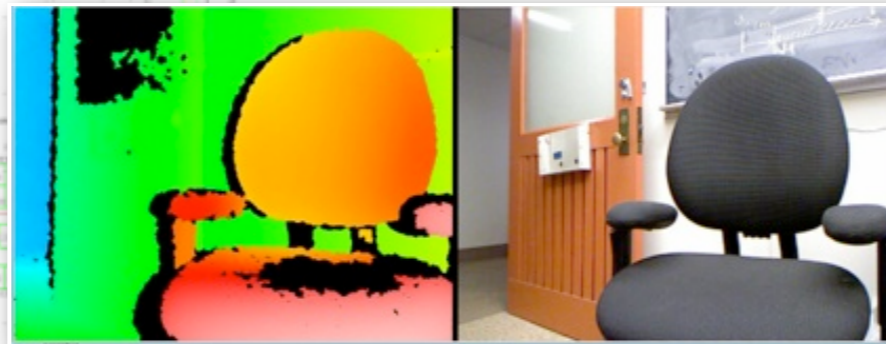
Real-time (30Hz) precise RGB-D image (color + depth) up to 5.5m distance, using the Kinect sensor
