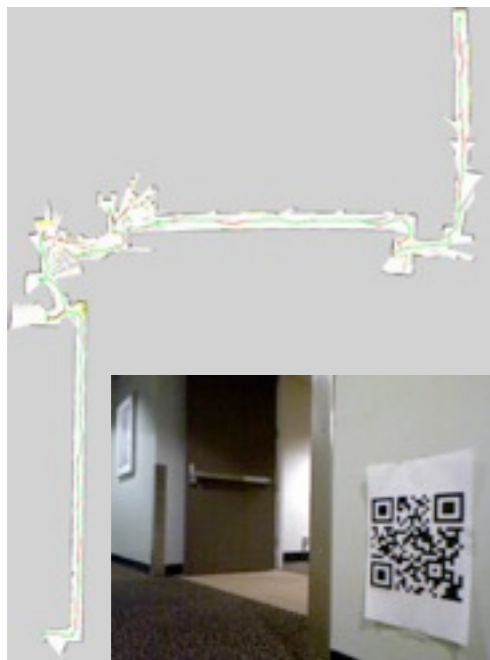
Simultaneous Localization and Mapping (SLAM) for map building from start (without blueprints), trajectory registration using self-describing QR codes
