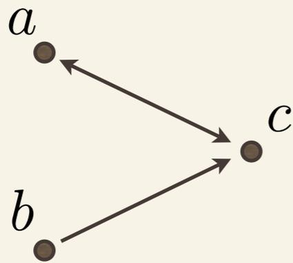
$(\bar{a} \vee \bar{b} \vee c) \wedge (\bar{c} \vee b)$
