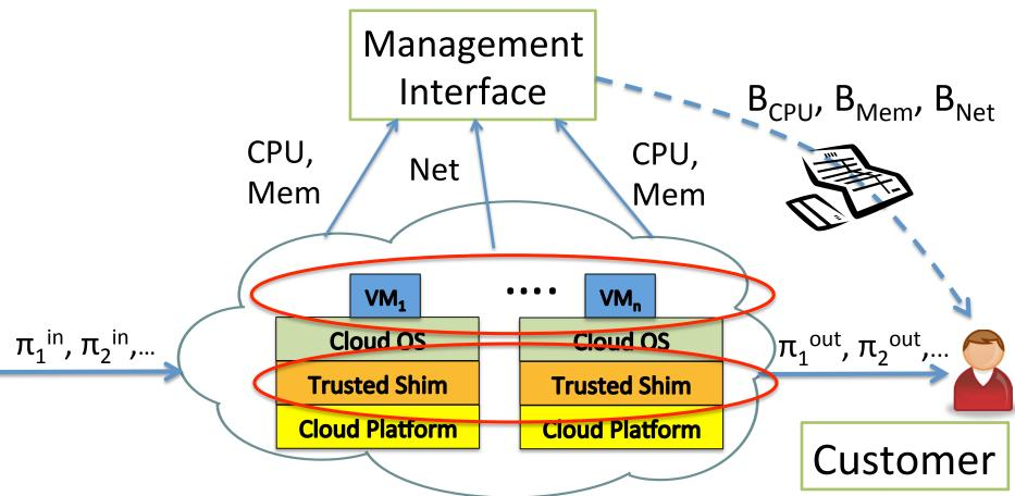
Each function is implemented as a virtual appliance. NFO provider deploys a trusted shim for logging.
