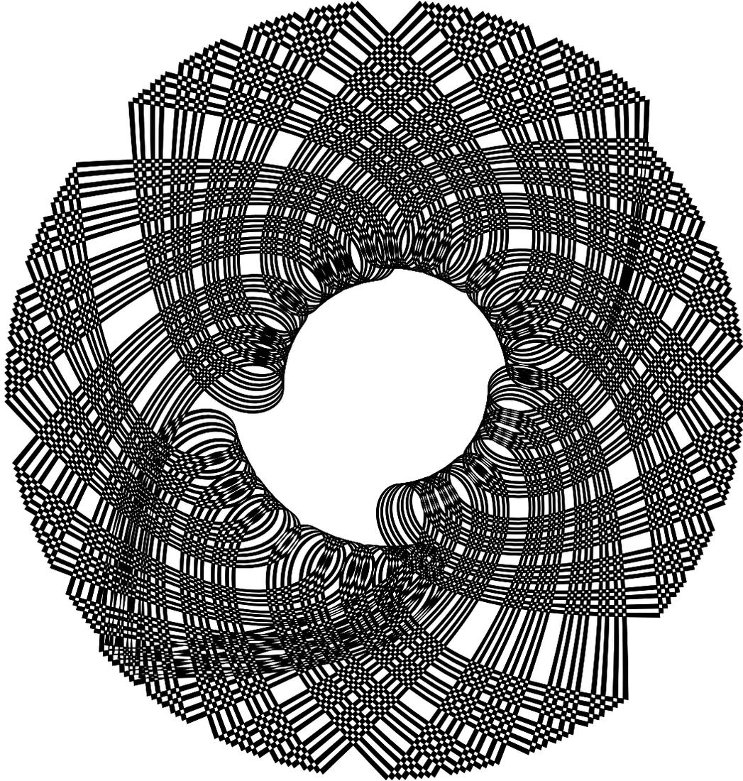
Figure 1: Region bounded by implicit cubic curve, rotated and XORed with itself 8 times, each rotation half the one before. Number of vertices = 23971, edges = 47185, and cells = 23216.
