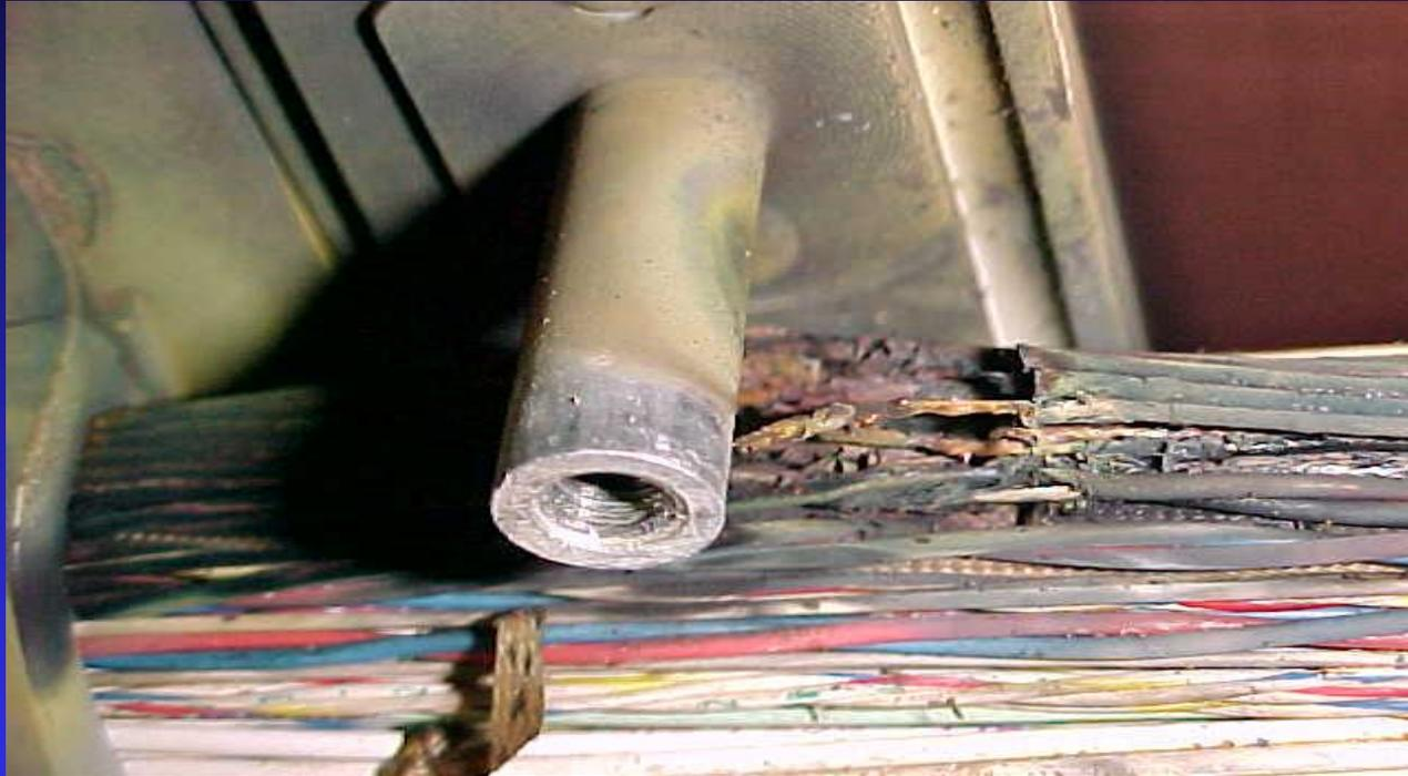
An arcing event has occurred. It is assumed that the arcing event began with one or two wire chaffing against the standoff. However, as a result of the arcing many wires in the bundle have failed. The possible effect of the failure depend on which systems are routed in the bundle.
