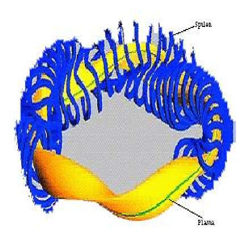
Tokamaks are axially symmetric, but the poloidal field is produced by transformer induced plasma current, pulsed, not steady state. First high energy plasmas were achieved with tokamaks in USSR. Initial attempts at Princeton were with stellarators and leaked, only low temperatures. But with new computer simulation capabilities designs can overcome the leakage. Wendelstein 7X - construction in Greifswald, Germany, **PLASMA 2015.**
