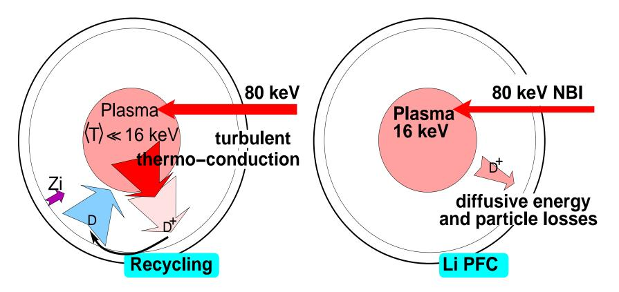
Plasma column heated by 80 KeV Neutral beam injection. High recycling as in present devices, T small at edge, large gradient. A pumping wall, utilizing liquid lithium and making the wall invisible to the plasma, giving small temperature gradient, low turbulence. Some experiments in Princeton, Intensly pursued in China. Success woud dramatically reduce size and cost of a reactor.
