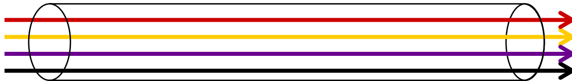
WDM fiber with 4 wavelengths.
