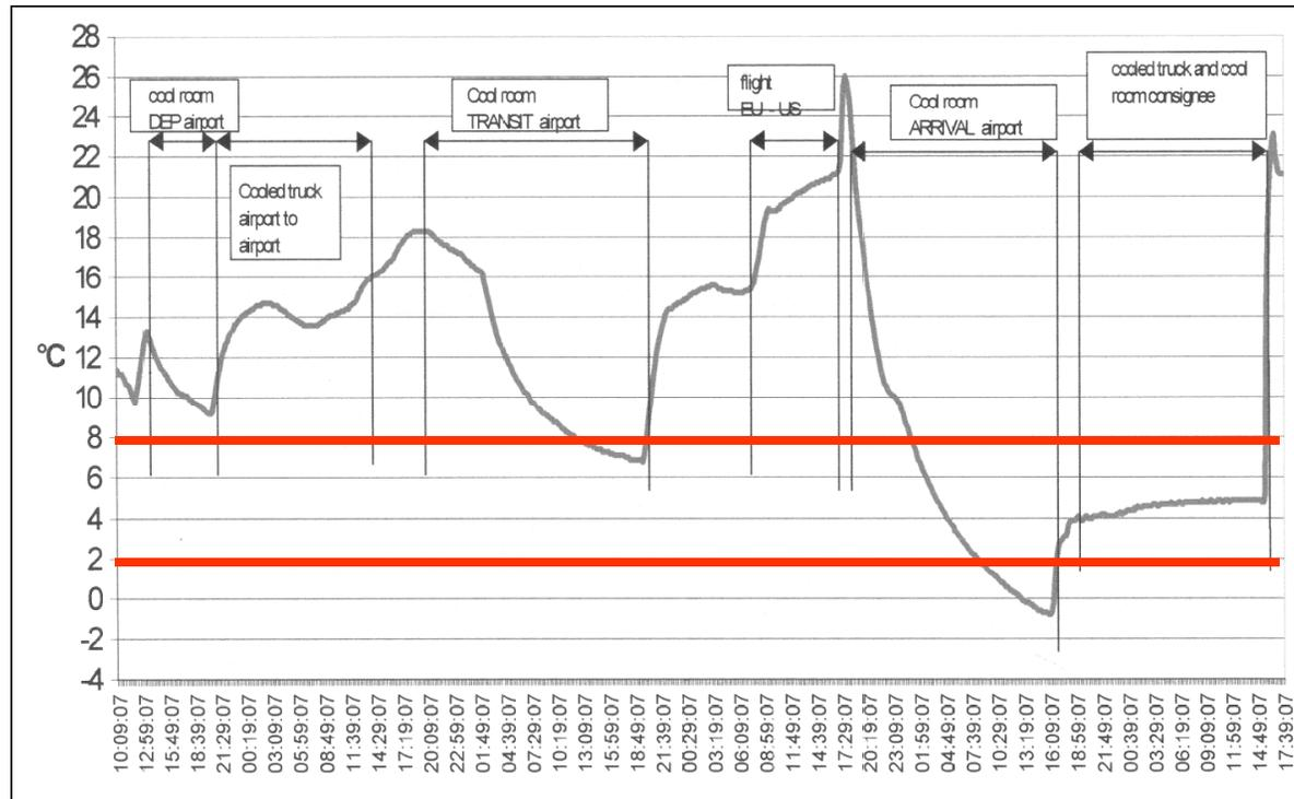
Temperatures in an air freight shipment with the instruction to maintain temperatures between 2 °C and 8 °C (Heap, 2006)
