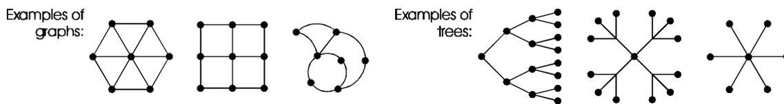
In the left-most graph of the figures above, all seven dots are linked into a network consisting of the six line segments emerging from the center dot; these six line segments form the tree at the far right which is said to “span” the original graph since it reaches all of its points. Another example: if we think of the second graph as a street map and we make the streets one way, we can represent the situation using a directed graph where the line segments are replaced by arrows.
